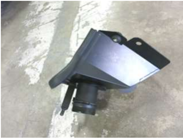
d. Assemble the passenger side intake system as shown. Take care to use the correct MAF housing bracket (part number "7-362" will be stamped on).
