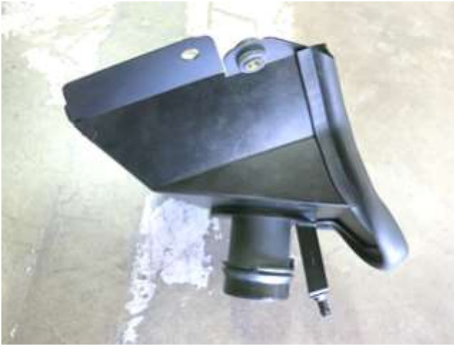
c. Assemble the driver side intake system as shown. Take care to use the correct MAF housing bracket (part number "7-363" will be stamped on).
