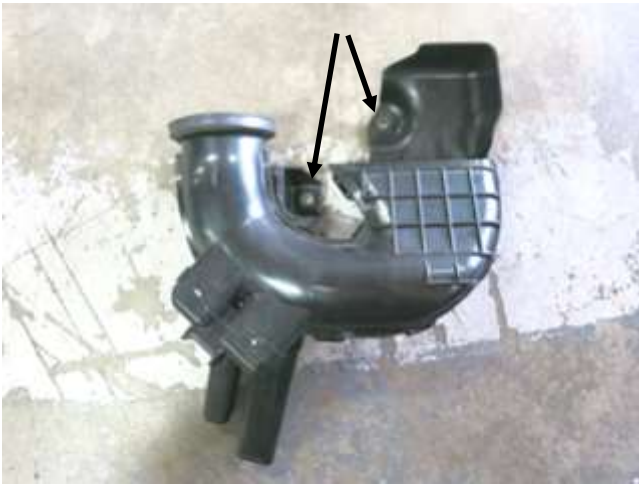
k. The positions of the two bolts from step 2j as seen from the front of the car are shown by the arrows. The left-hand side bolt will require a short extension. Allow the resonator to fall to the bottom of the bumper area once both bolts are removed.
