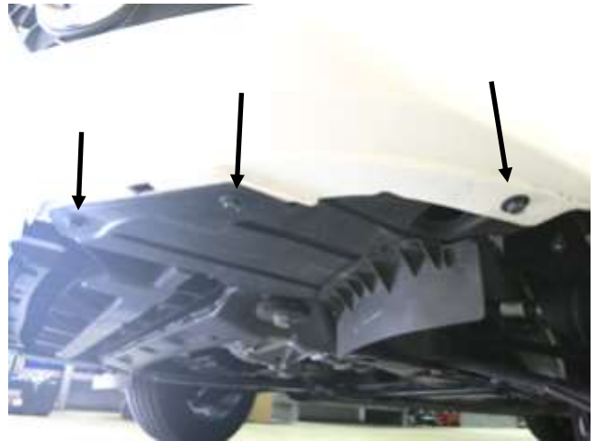
n. Remove the three bolts securing the front of the inner fender liner.
