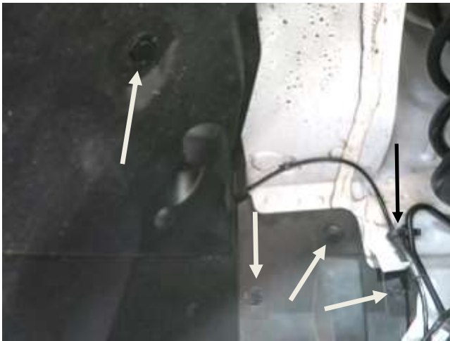
m. Remove the 4 plastic push-in clips in the fender well area indicated. The ABS wire will need to be moved for access (black arrow).
