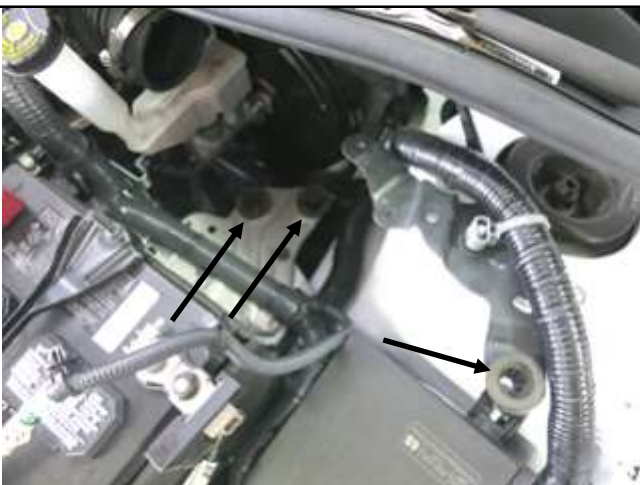
i. Remove the three grommets from the engine bay and store them on the air box for safe keeping. They will not be reused.
