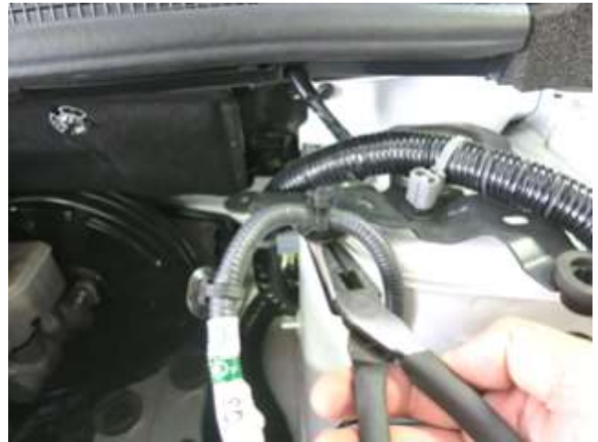
h. Release the metal wire from the metal bracket as show and move the MAF harness down and out of the way.
