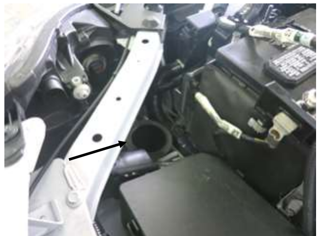
j. Use the next picture to help in removal of the intake resonator indicated in this step. Both bolts are accessible from above using a ratchet, socket, and extension.
