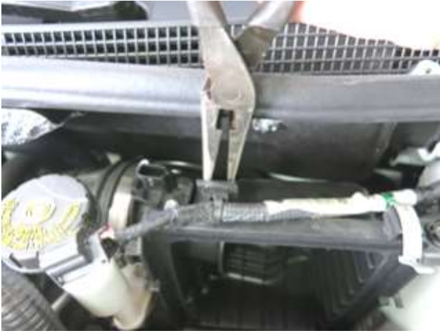
e. Disconnect the Mass Air Flow (MAF) sensor harness. Release the harness from the air box using pliers as shown.
