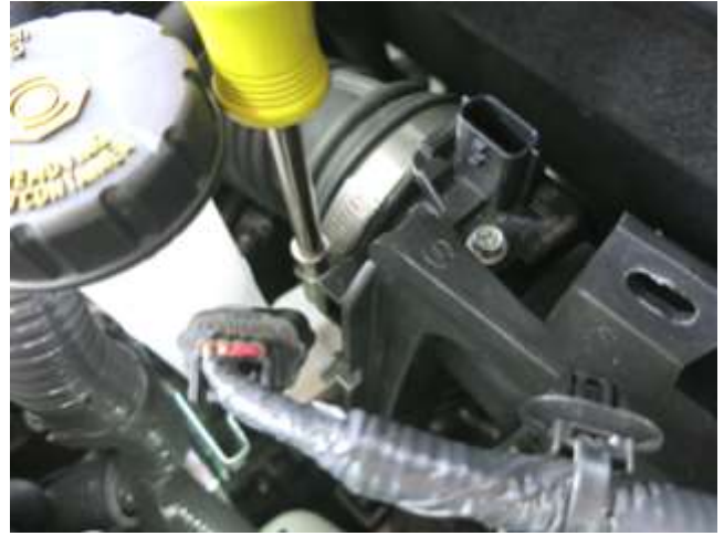
f. Loosen the hose clamp securing the factory coupler to the air box.
