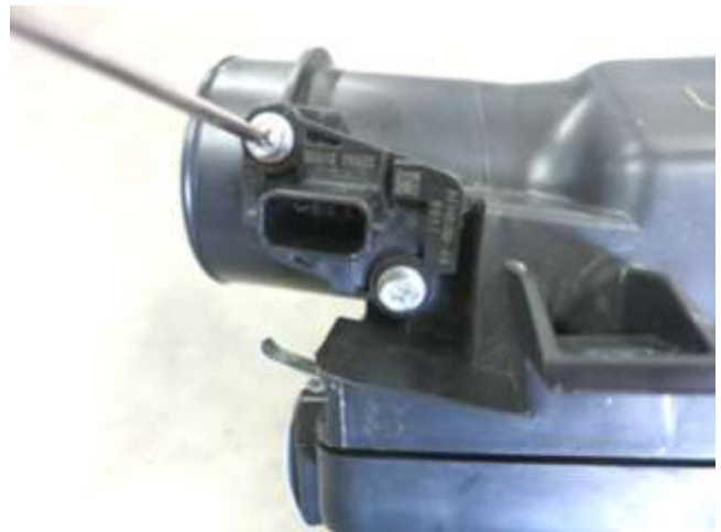
p. Remove the MAF sensor from the factory air box. The MAF sensor and screws will be reused in step 3b.
