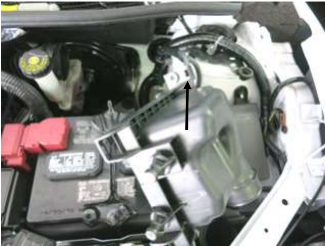
g. Pull up on the air box to release it from its grommets, disconnect the coupler, and turn the box on its side as shown to access the next wire. Release the harness from the air box and remove the air box from the engine bay.
