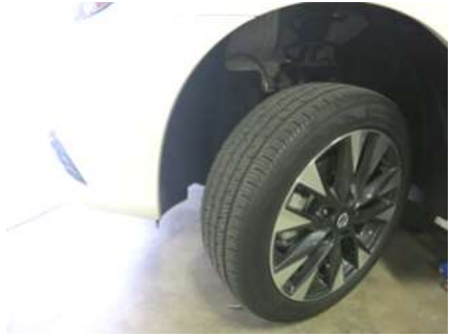
l. Lift the front of the car with a jack and turn the wheels to the left. Note: Support car with jack stands once lifted.
