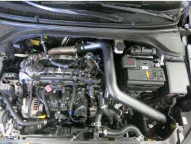
c. Install the AEM intake tube into the coupler, then attach the tube to the 6mm rubber mount with supplied M6 nut and washer. DO NOT TIGHTEN THE BAND CLAMP UNTIL FILTER IS INSTALLED.
