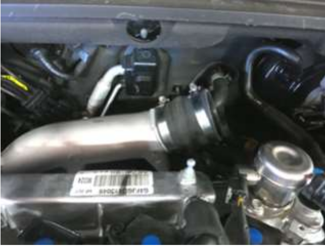
a. Install the supplied coupler and the 2 #44 band clamps. Tighten the turbo tube side only.
