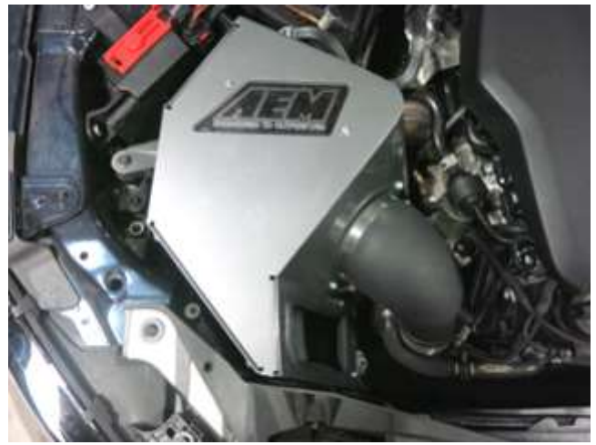
l. Place the air box into the engine bay. Align the [3] push-in studs and make sure they seat into their respective grommets. Make sure the coupler is fully seated onto the turbo inlet then tighten both hose clamps.
