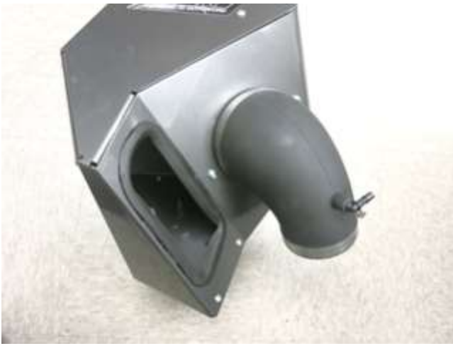
k. Loosely install the coupler with hose clamps. Then install the vacuum hose to the coupler.
