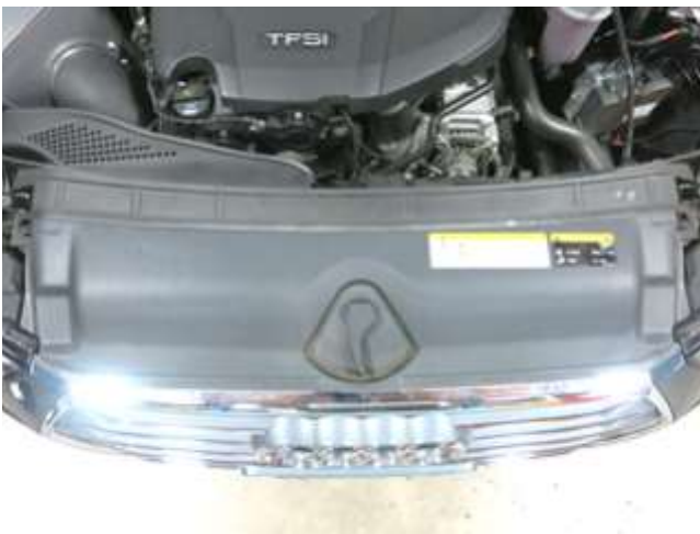
o. Finally, reinstall the radiator shroud and hood release latch.
