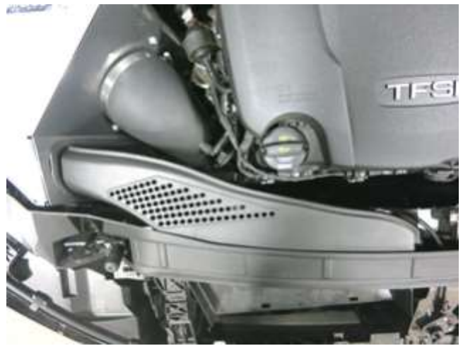
n. Reinstall the inlet scoop. Slide the scoop into the rubber gasket first then align with the core support. Secure with the [2] T25 Torx bolts removed in step 2c.
