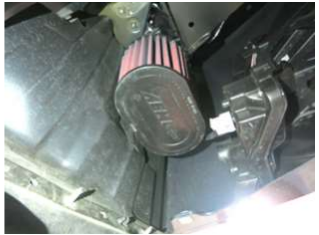
h. Install the air filter onto the tube. Be sure to have clearance around the filter before tightening the clamp.
