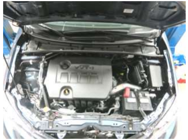
AEM INTAKE INSTALLED
