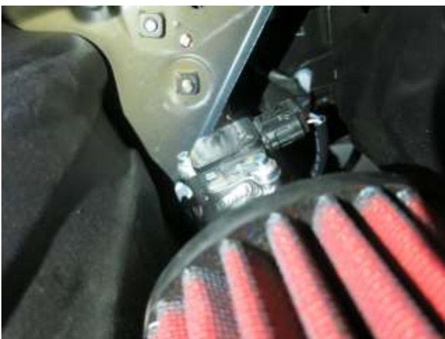
i. Connect the MAF harness extension to the MAF sensor. Then, reinstall the 2 bolts and push clip to secure the fender liner pulled back in step 3f.
