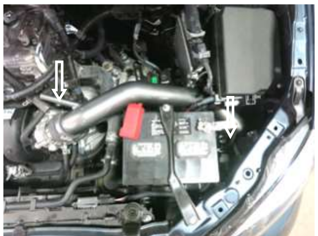
j. When proper tube alignment and clearance is achieved, tighten the m6 nut on the rubber mount and the hose clamp on the throttle body and reinstall engine cover.
