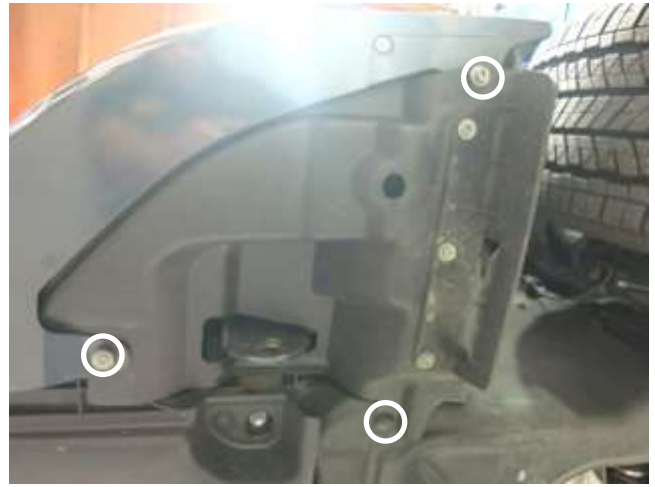
f. Lift the vehicle up with floor jack and secure it with jack stands. Remove the 2 bolts and the push clip on the fender liner as shown. Then pull back fender liner for access.
