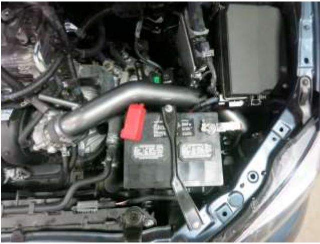
e. Secure the battery by tightening the bolt on the core support, then tighten the nut on the battery strap.
