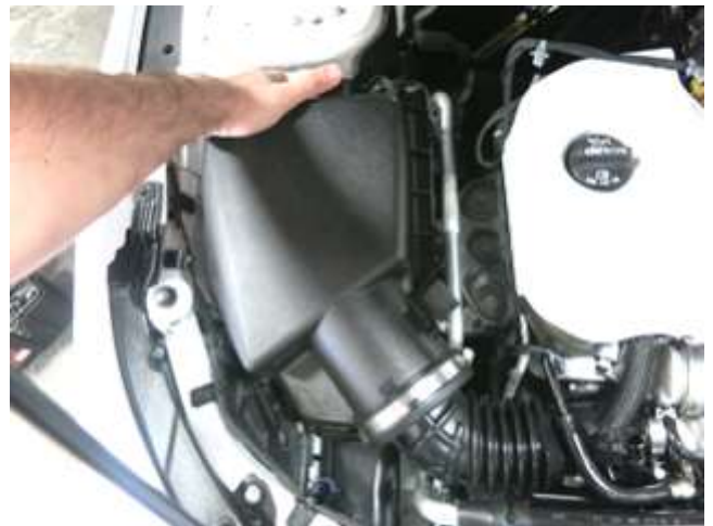
d. Release the air box from its rubber grommets by pulling up gently on the air box as shown.
