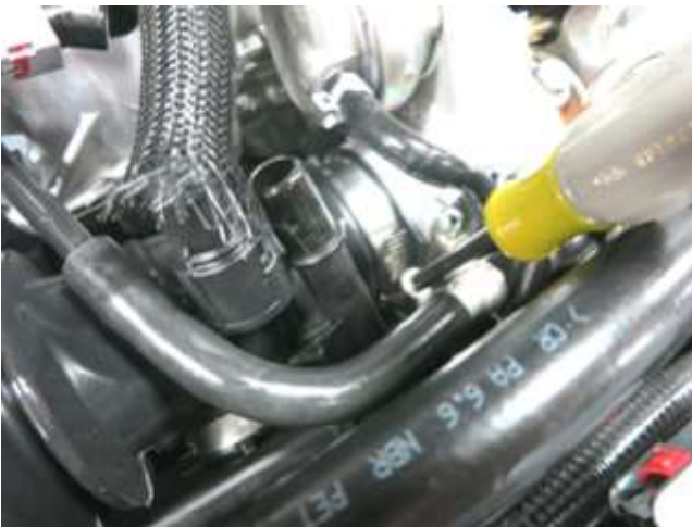
c. Loosen the hose clamp at the turbo side of the factory air hose.
