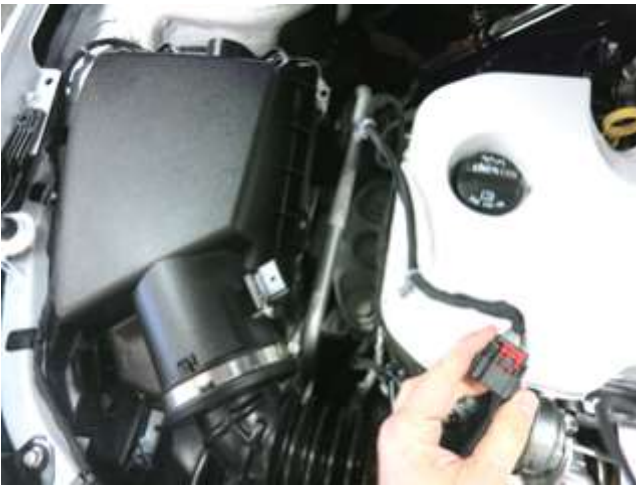
a. Disconnect the Mass Air Flow (MAF) sensor connector and harness ties from the sensor and air box.
