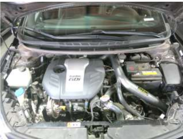
o. Install the engine cover by aligning the post to the rubber grommets, then pressing down until they are seated.
