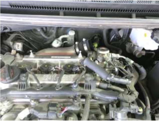
a. Install the supplied coupler and the 2 #44 band clamps.
