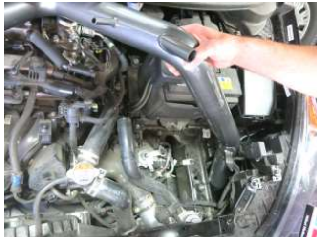
d. Pull the filter end up and over the frame rail to its proper place in the front wheel well.
