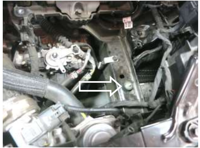
b. Install the 6mm rubber mount in the stock air box mounting hole.
