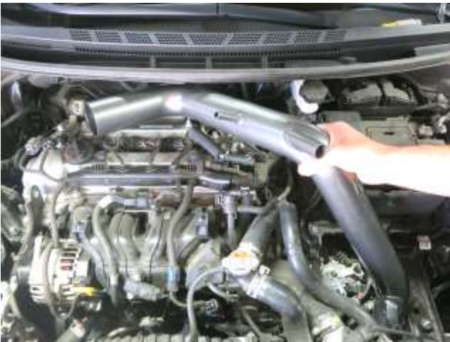
c. Install the AEM intake tube by dropping the filter end inside the frame rail first, then swing the turbo inlet side in towards the fire wall.
