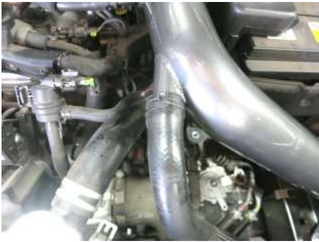
n. Reinstall the recirculation hose to the intake tube and secure using the stock spring clamp.
