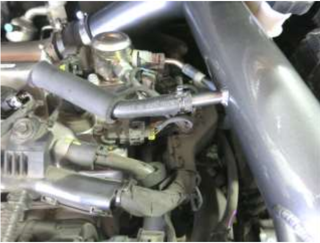
m. Reinstall the PCV hose to the AEM intake tube and secure using the stock spring clamp.
