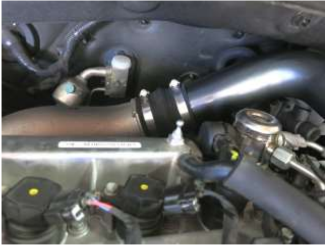
l. Properly align the intake to make sure there is clearance, then tighten the 2 band clamps with an 8mm nut driver. Torque spec: 30in-lb
