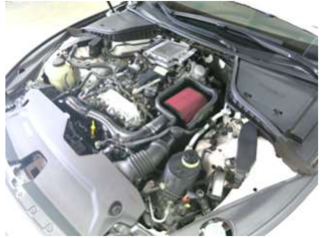
AEM INTAKE INSTALLED (ENGINE COVER REMOVED)
