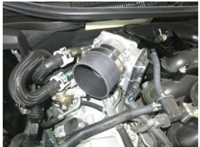
d. Install the provided coupler and hose clamps onto the throttle body. Tighten the hose clamp closest to the throttle body at this time. Move the tube-side hose clamp as close to the throttle body as possible to allow room for tube installation.
