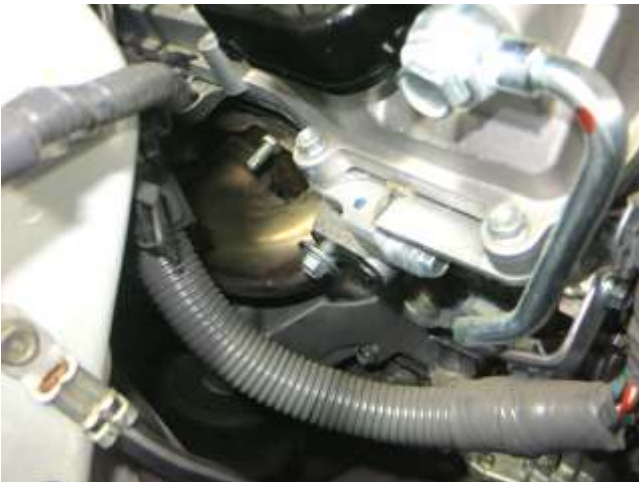
c. Thread the included large bolt and washer onto the location shown on the side of the motor. Leave roughly 1/4" of space for the intake tube bracket.
