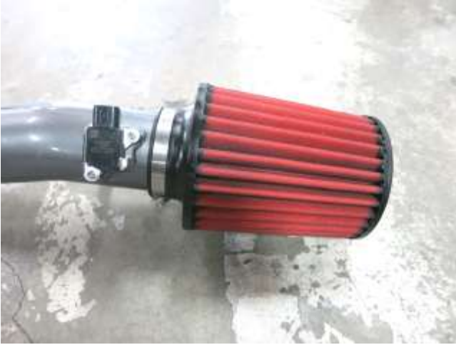
a. Install the MAF sensor using the supplied bolts, then install the AEM DryFlow filter using the supplied hose clamp.
