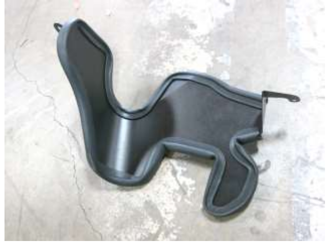
b. Apply the edge trim to the heat shield as shown.
