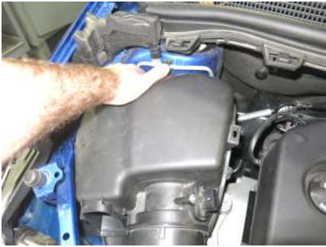
f. Release the air box from its rubber grommets by pulling it up and out of the engine bay while disconnecting the intake hose from the turbo.
