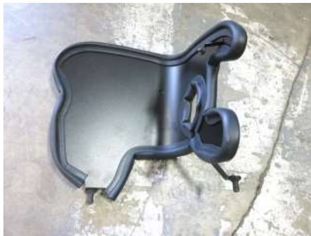
b. Install the hardware and edge trim to the heat shield as shown. Note: Some trimming of the edge trim will be required.
