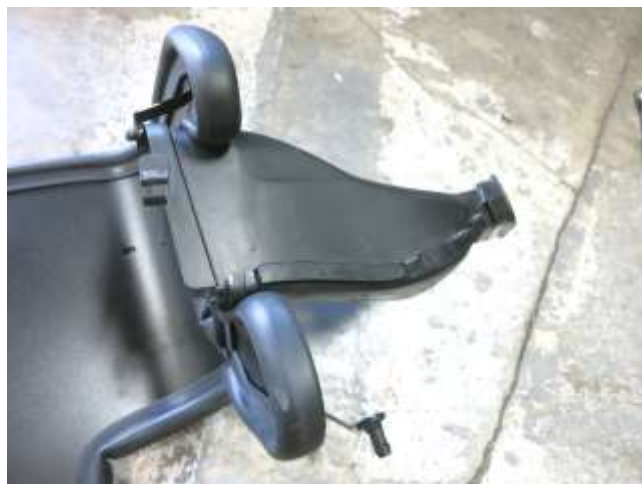
d. Carefully insert the cold air duct into the cut out in the heat shield as shown by rotating it into position. Ensure the tab and grommet are retaining the duct as intended.
