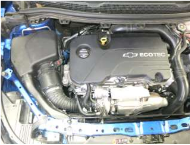
STOCK INTAKE INSTALLED
