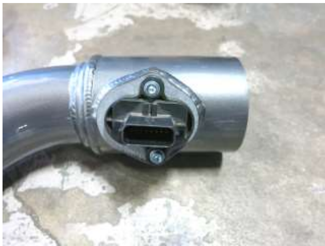
a. Install the MAF sensor into the AEM intake tube using the provided screws and washers.
