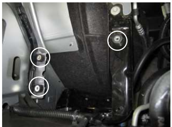
h. Install the three supplied bushings and mount them into the inner right side fender.
