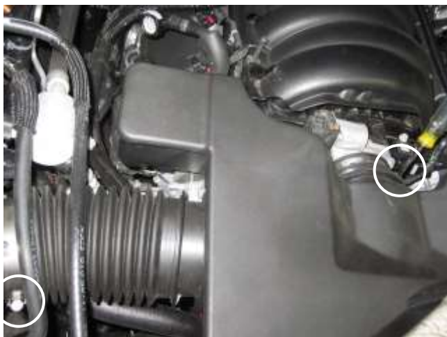
c. Loosen the hose clamps on the air box and the throttle body. Then pull the resonator box out of the vehicle.
