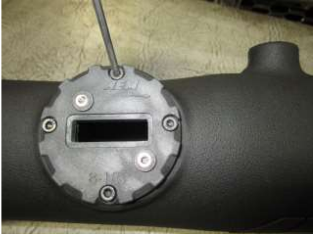
b. Install the mass air sensor adapter onto the tube with the provided M4 allen bolts.
