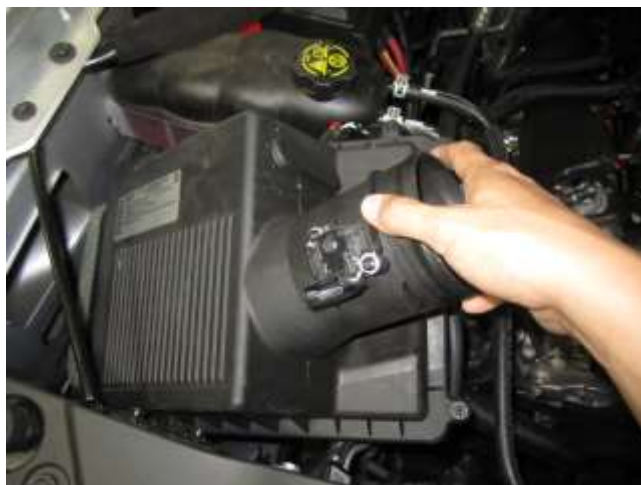
d. Gently pull up on the air box to remove it from the rubber grommets and remove from engine compartment.
