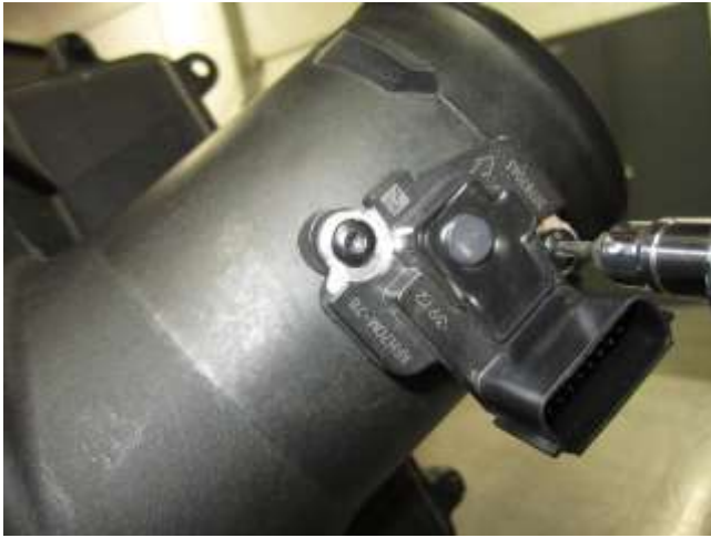
f. Remove the two M4 torx bolts with a T15 bit and slide the mass air sensor out of the tube. Note: Be very careful with the sensor. This will be re-installed in step 3c
