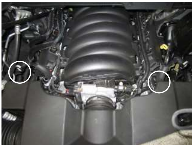
a. Remove both crankcase vent hoses by squeezing the white clip at the valve cover breather port.
