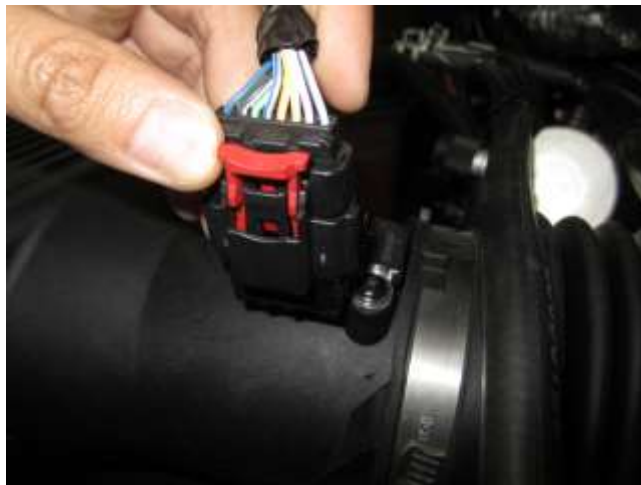
b. Pull up on the red locking clip, then depress down on the black tab while removing the mass air sensor connector.
