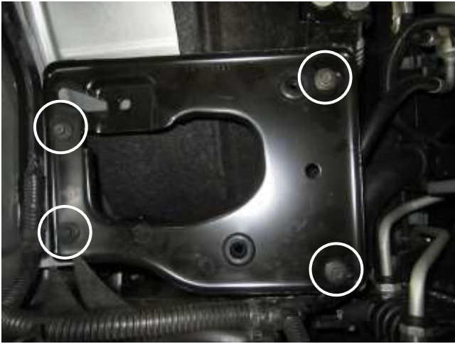
e. Loosen and remove the four M6 bolts. Remove the air box plate from the vehicle. These will not be re-used. Note: Do not discard the plate or hardware.
