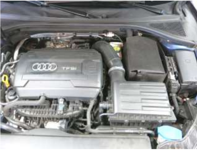
STOCK INTAKE INSTALLED
