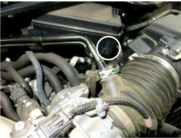
c. Squeeze the spring clamp and remove the vent line from the stock intake duct. This will be reused in step 3f.
