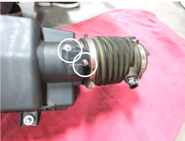
m. Remove the two screws securing the MAF to the stock air box. These will be reused in step 3c.
