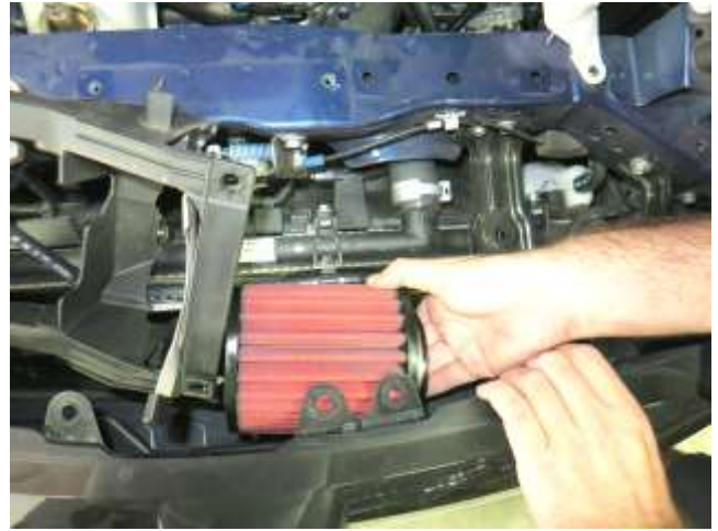
b. Rotate and move the plastic bracket you unfastened in step 2i, so that you can place the air filter in between the radiator and grill as shown.
