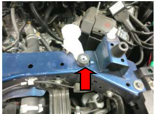
d. Use a 10mm socket and ratchet to remove the bolt holding the coolant overflow tank neck to the upper core support. Replace the bolt with the supplied rubber mount as shown.
