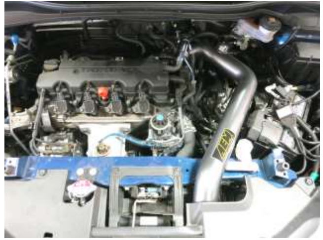
AEM INTAKE INSTALLED
