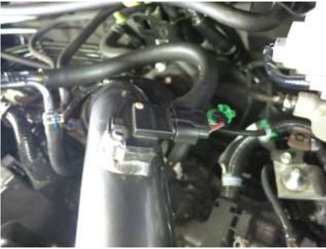
l. Reconnect the MAF sensor harness.
