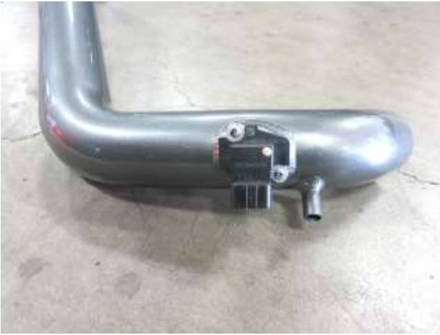
a. Install the MAF sensor you removed in step 2j onto the AEM intake tube as shown using the same hardware.
