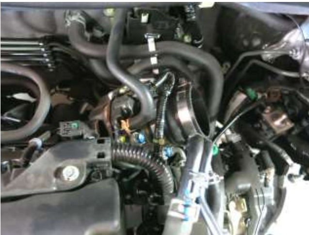
c. Place the AEM throttle body coupler with the 2 hose clamps onto the throttle body. Tighten the hose clamp closer to the throttle body to 30 in-lbs. Leave the other hose clamp loose. You will fully tighten this in step 3m.
