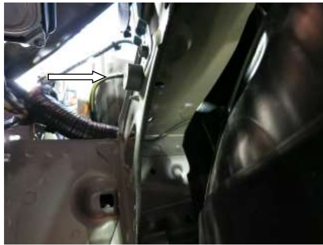
h. On 2015 and earlier models, Install the female to male rubber isolated onto the inner fender as shown. See step 3j for directions for 2016 and newer models
