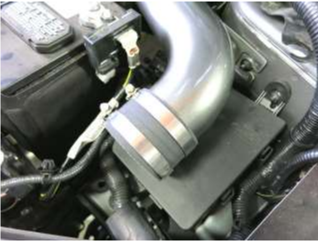
e. Install the coupler to the end of the AEM upper intake tube as shown.
