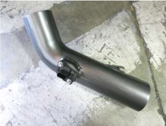
a. Install the MAF sensor into the AEM lower intake tube using the screws removed in step 2p.
