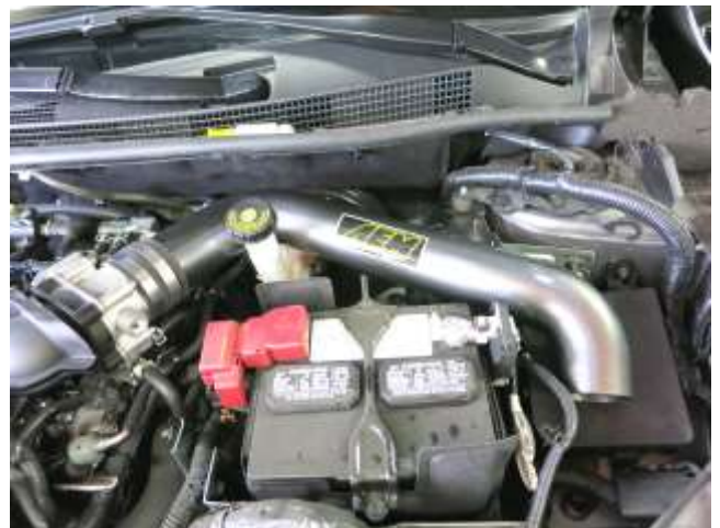
d. Install the AEM upper intake tube as shown and secure the bracket to the isolator using the nut and washer provided.
