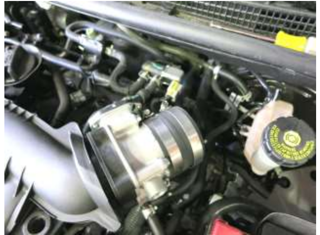
b. Install the provided coupler and hose clamps onto the throttle body. Torque the throttle body side hose clamp to 30 in-lbs at this time.
