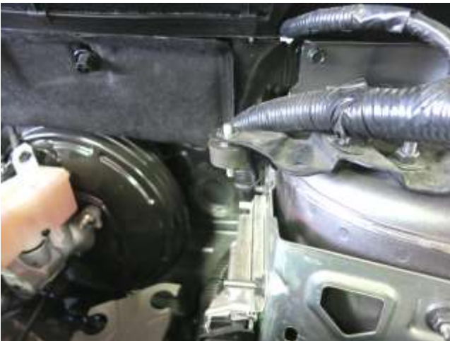
c. Thread the male-to-male rubber isolator mount to the underside of the air box mount as shown.
