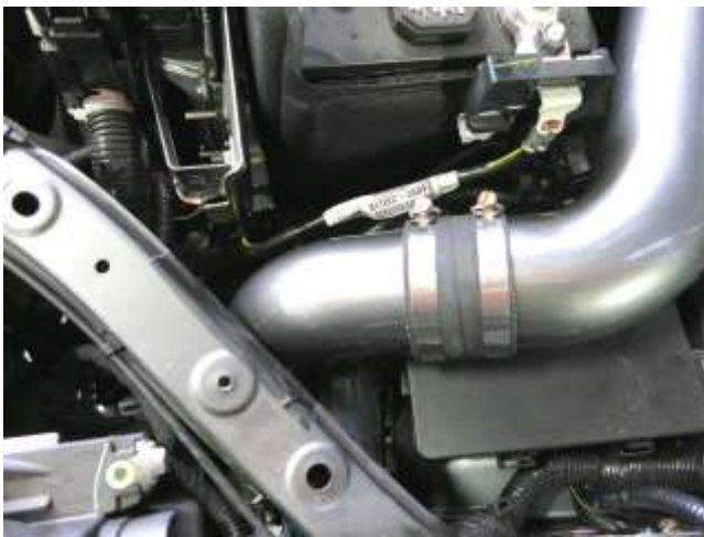
i. Install the AEM lower intake tube from the bottom of the car.
