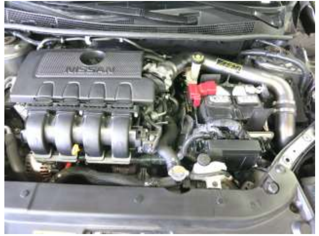
AEM INTAKE INSTALLED
