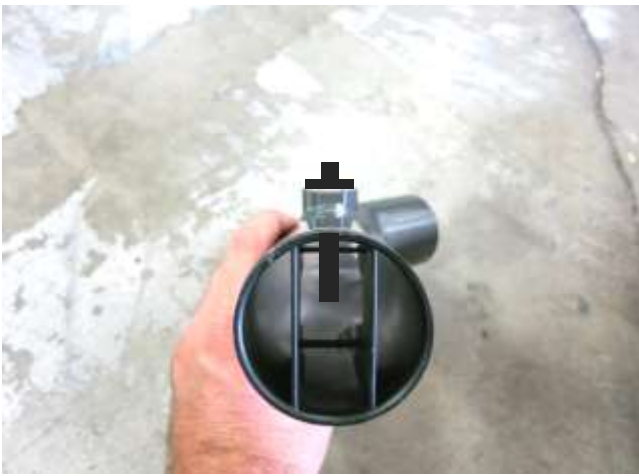
g. Quickly install the air straightener into the long end of the AEM lower intake tube aligning the vanes with the MAF sensor as shown. Refer to the exploded view for clarification.
