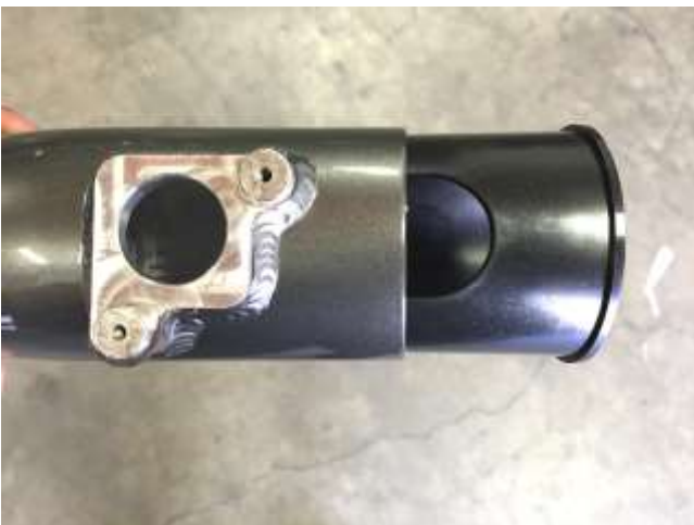
d. Install the venturi all the way into the tube in the orientation shown above.
