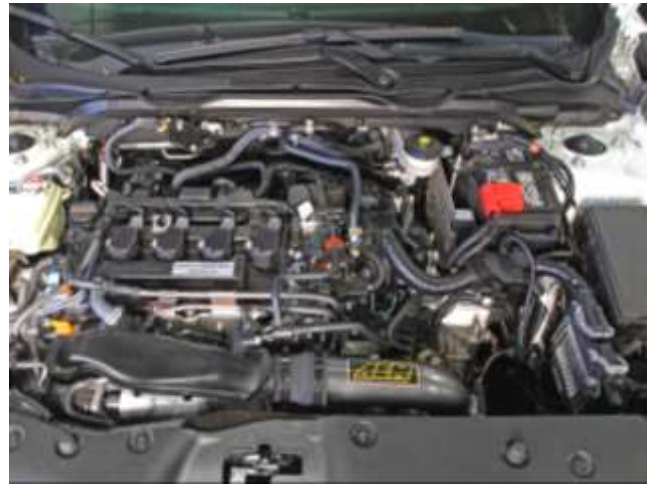
AEM INTAKE INSTALLED
