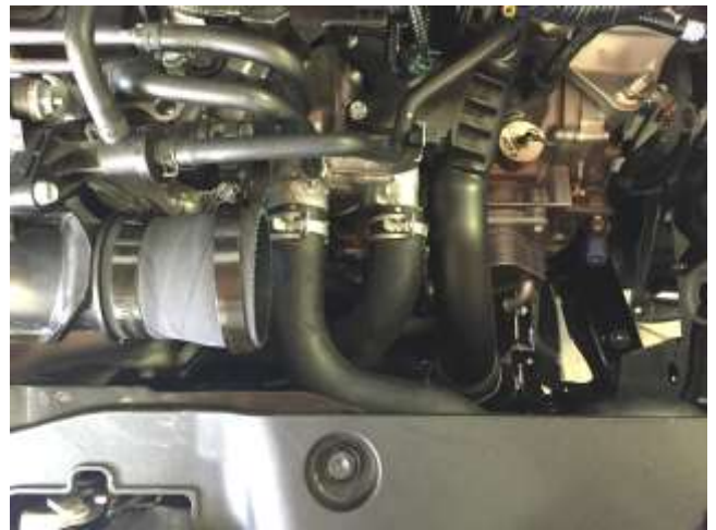
c. Install the upper hose and clamps. The leftmost clamp may be tightened to 30 in-lbs at this time.
