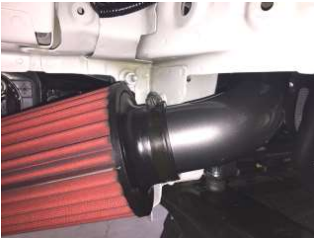
b. After loosely assembling the filter, cold-air tube, 5-275 hose, and corresponding hose clamps, maneuver the tube into place from the fender-well and position the bracket loosely in the rubber mount. Torque the filter hose clamp to 30in-lbs. The fender liner and undercarriage opened in steps 2d and 2e may now be reinstalled in reverse order from how they were removed.
