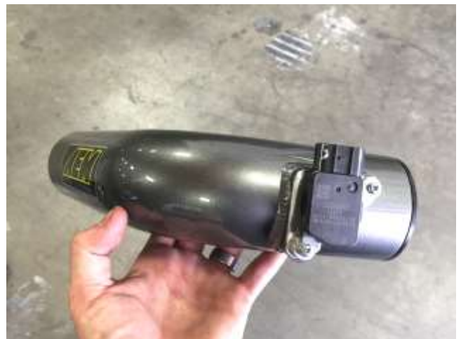
e. Remove the MAF sensor from the OE air box and install it into the short ram tube using the factory screws.
