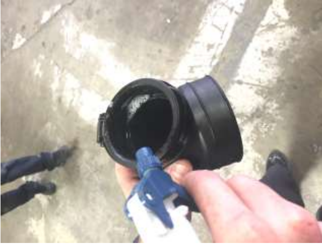
a. Install the small end of included coupler with it's corresponding hose clamps on each end (refer to diagram on pg2). Using soapy water as a lubricant is helpful.
