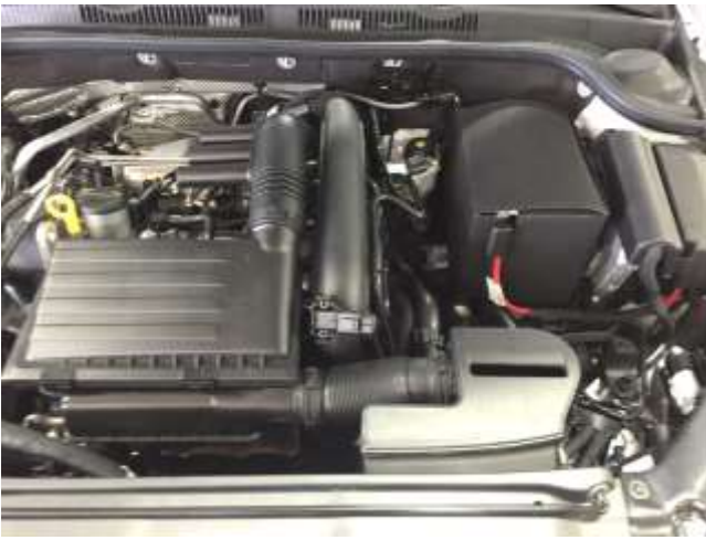
STOCK INTAKE INSTALLED
