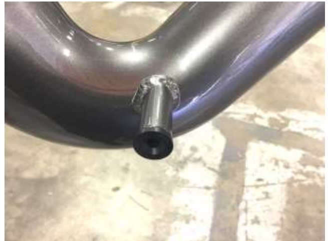
d. Press the factory grommet removed in step 2d into the stand-off on the bottom of your new AEM intake tube. Again, using soapy water as a lubricant may be helpful.
