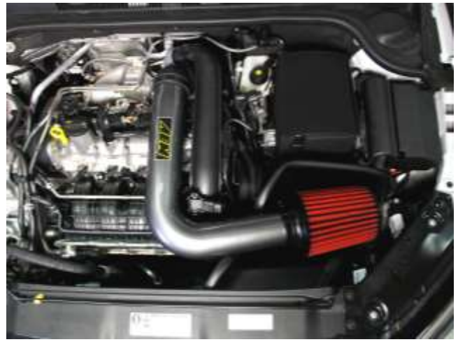
AEM INTAKE INSTALLED
