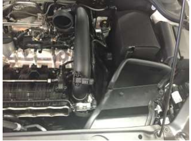
b. Assemble the heat shield assembly including the edge trim & grommets as shown in the diagram on pg 2 & install as shown. Cut off excess trim if necessary.
