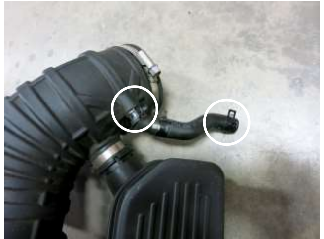
l. Remove the two outside spring clamps off the stock intake vent line. Note: These will be reused in step 3k.
