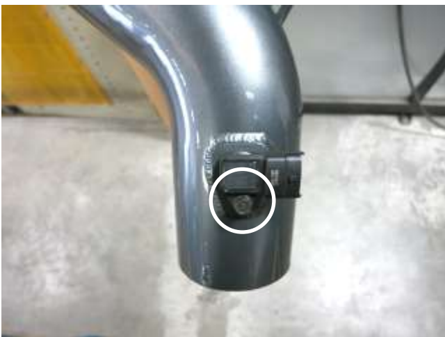
a. Install the pressure sensor with the bolt removed in step 2m into the AEM intake tube.
