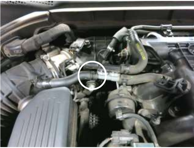
e. Release the tension on the spring clamp, and remove the hose from the 2-way check valve.
