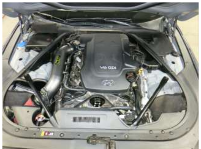
AEM INTAKE INSTALLED
