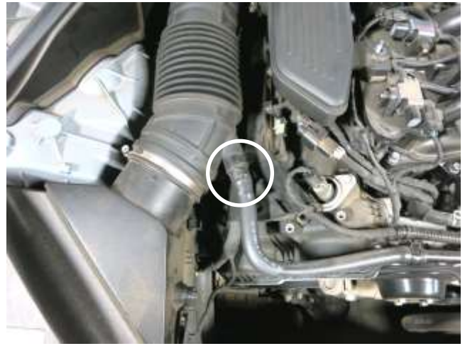
f. Release the tension on the spring clamp, and remove the hose from the stock intake tube.
