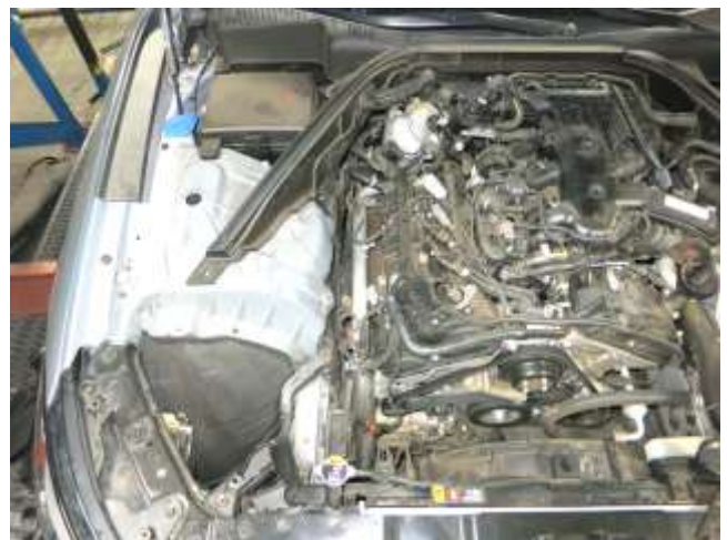
j. Remove the stock intake assembly by lifting it up and out of the vehicle.
