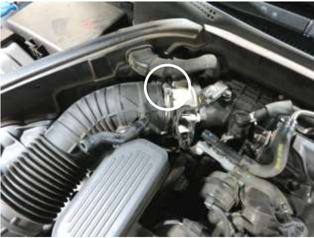
g. Loosen the hose clamp at the throttle body.
