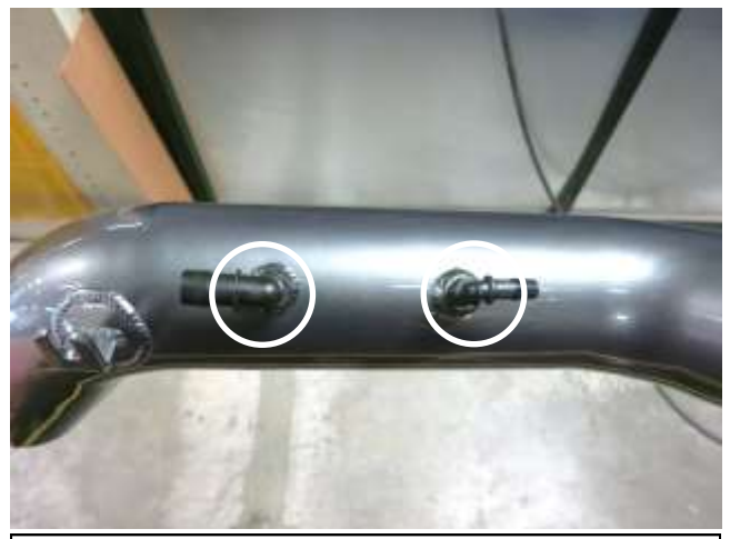
b. Install the provided 90° elbows into the AEM intake tube as shown. Note: The larger one will go on the filter side of the AEM intake tube.
