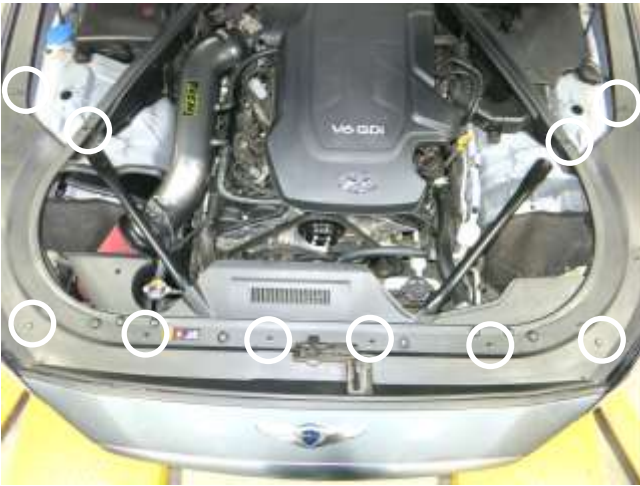
n. Reinstall the engine bay cover into the vehicle and secure with the clips removed in step 2a. Note: You will only use 12 of the clips (not all pictured)
