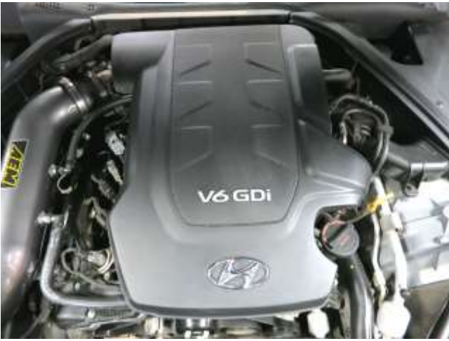
l. Reinstall the engine cover that was removed in step 2b. by aligning the 4 mounts to its grommets.
