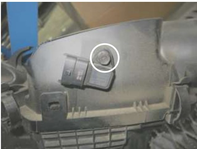
m. Remove the bolt securing the pressure sensor to the stock upper air box. Note: this will be reinstalled in step 3a.
