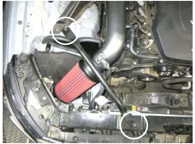
m. Reinstall the brace and bolts onto the vehicle and tighten to 3.6 ft-lbs.
