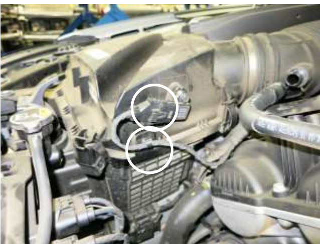
i. Remove the pressure sensor connector from the sensor, then unclip the harness from the air box.
