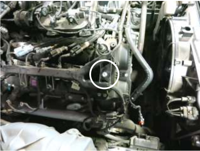
k. Remove the bolt circled on the passenger side valve cover. Note: This will be reused in step 3j.
