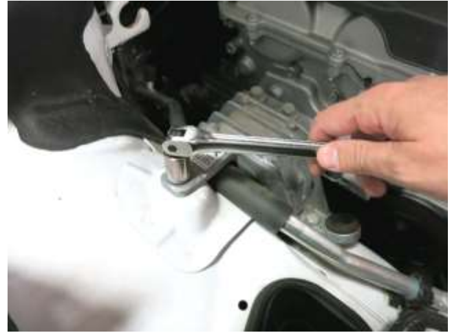
h. Loosen and remove the 15mm bolt on the engine mount. The bolt will be reinstalled in step 3f.
