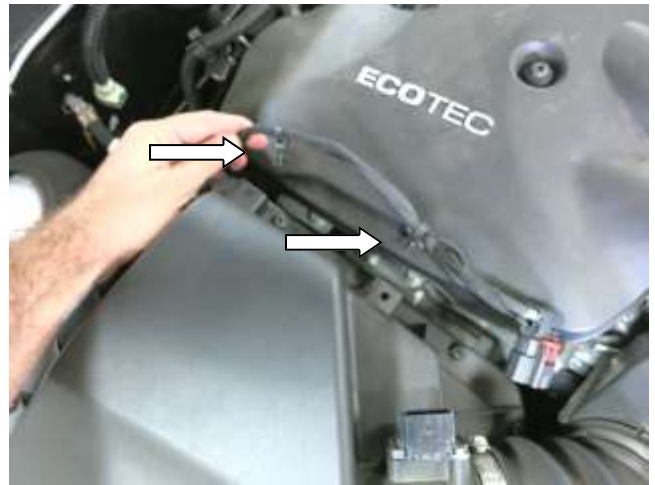
b. Release the MAF sensor wiring harness clips from the air box.
