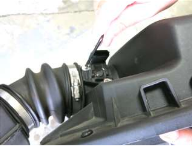
g. Loosen the MAF sensor screws and remove the sensor from the air box. The sensor will be reused in step 3a.
