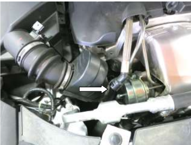
c. Release the quick-disconnect from the factory air intake tube. This will require using a thin flathead screwdriver to reach the clip.
