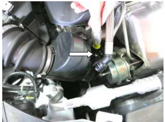
d. Loosen the hose clamp that secures the stock intake tube to the turbo.
