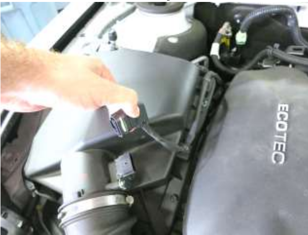
a. Unclip the red locking tab on the mass air flow (MAF) sensor connector to release the connector from the sensor.
