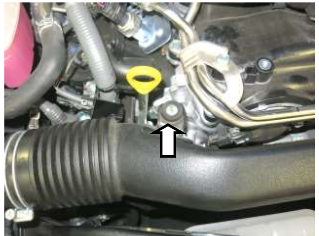
d. Remove the M6 bolt holding the intake tube to the engine.
