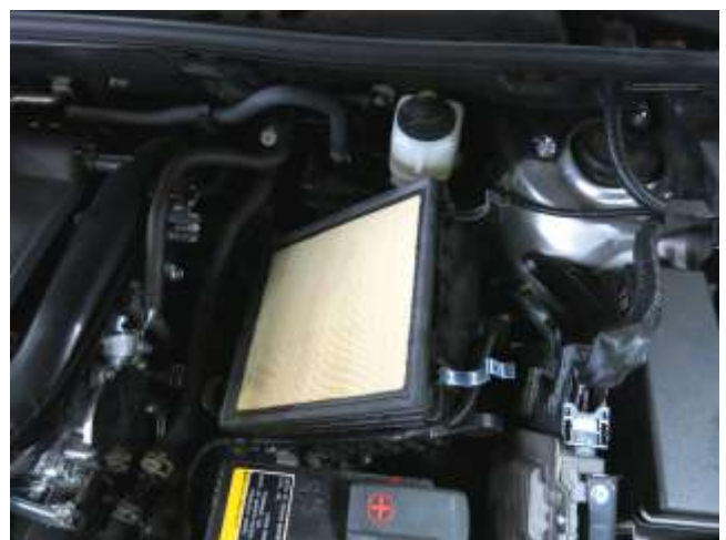
j. Remove the stock air filter from the lower air box.
