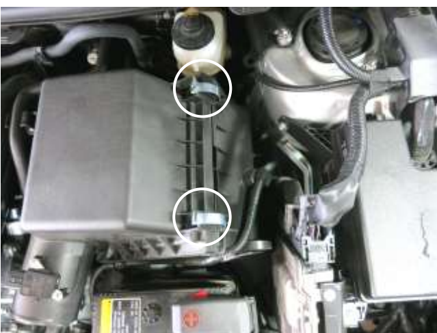
i. Unlatch the two clips that hold the upper air box to the lower air box and remove the upper air box.
