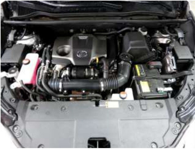
STOCK INTAKE INSTALLED
