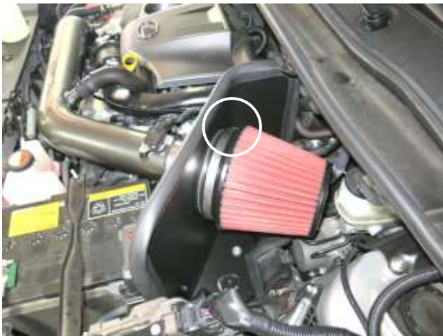
o. Install the AEM filter onto the filter adapter and tighten the hose clamp.
