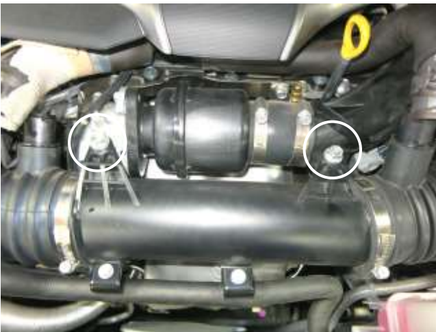
c. Loosen and remove the two bolts securing the stock intake tube to the vehicle.
