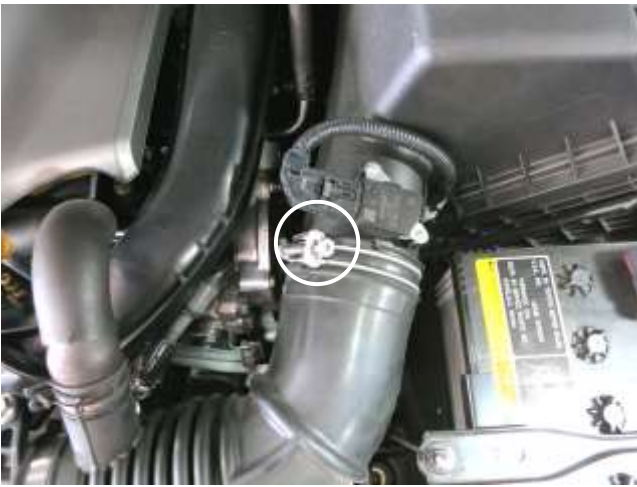
a. Loosen the hose clamp at the air box.
