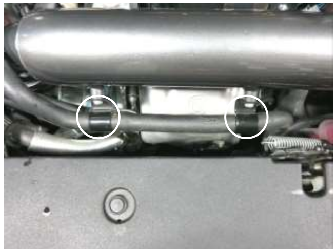
p. Place the hose back into the clips that were removed in step 2e.
