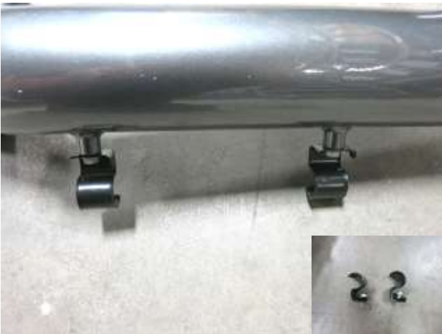
c. Take the stand-offs and bolts from step 2p. and install the bolts according to the inset picture. Then, install them onto the AEM intake tube as shown.
