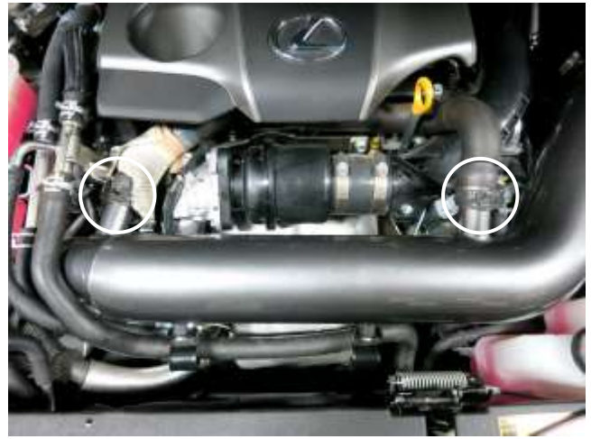
l. Install the vent hoses onto the AEM intake tube and secure with the spring clamps removed in step 2b.
