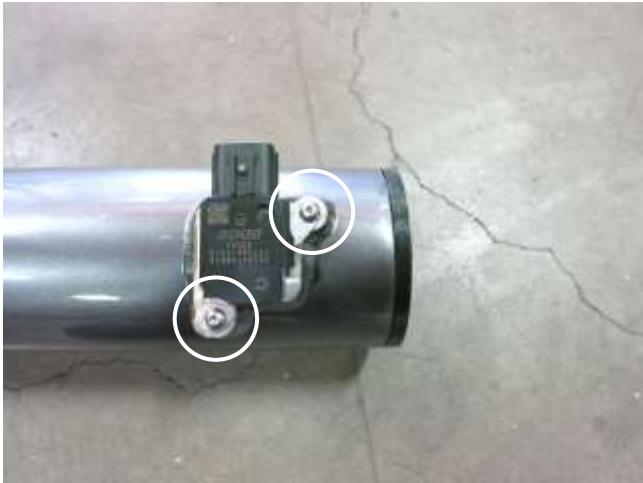
b. Install the MAF sensor into the AEM intake tube and secure with the provided hardware.
