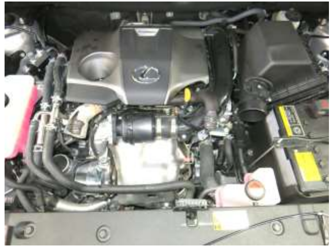
f. Remove the stock intake tube from the vehicle.
