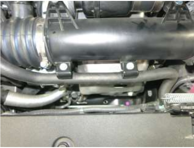
e. Slide the hose out of the clips that hold it on the stock intake tube.
