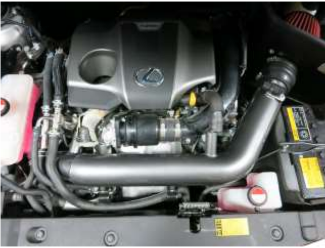
k. Install the AEM intake tube into the vehicle aligning the tube with the previously installed hoses.
