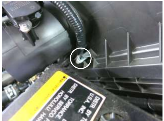
h. Slide the wire loom clip off of the air box.
