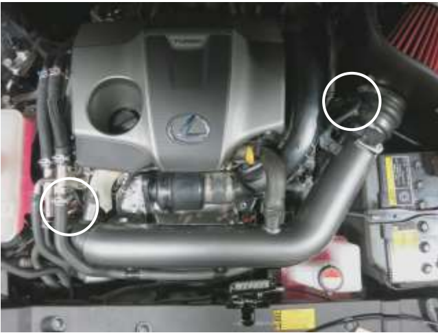
m. Tighten the hose clamps at the turbo compressor and heat shield securing the AEM intake to the hoses.
