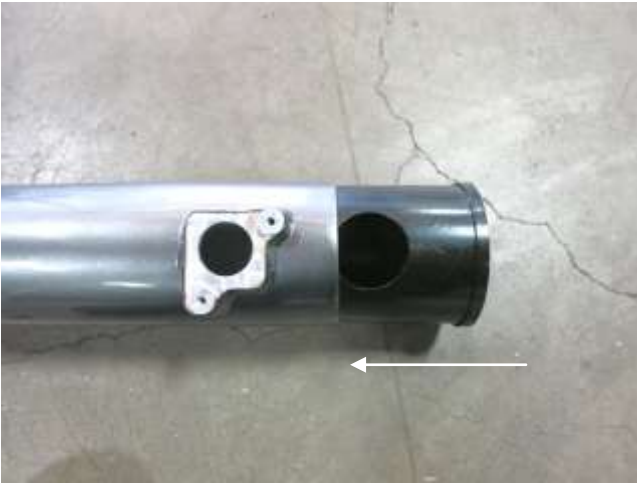
a. Install the venturi into the AEM intake tube, be sure the two openings are aligned.
