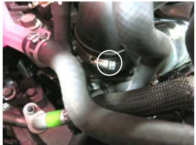
d. Loosen the hose clamp at the turbo compressor inlet.
