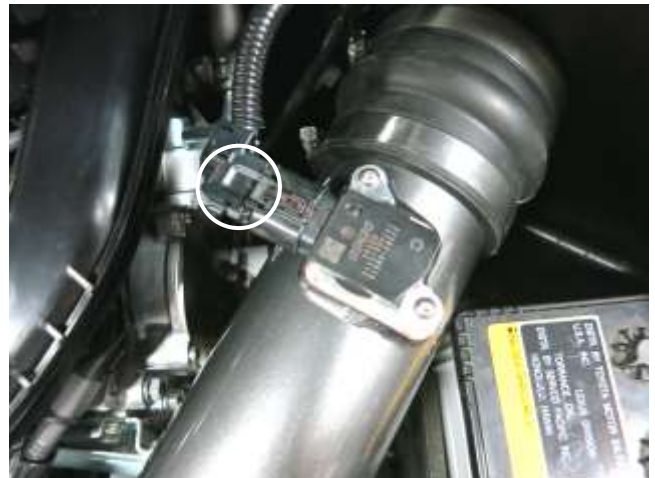
n. Plug the MAF sensor connector into the MAF sensor.
