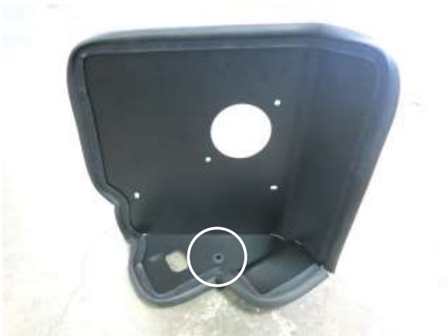
d. Install the edge trim as shown around the AEM heat shield, trim off excess if necessary. Then, install the provided grommet into the hole shown.
