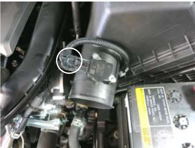
g. Depress the clip and remove the mass air flow (MAF) sensor connector from the sensor.
