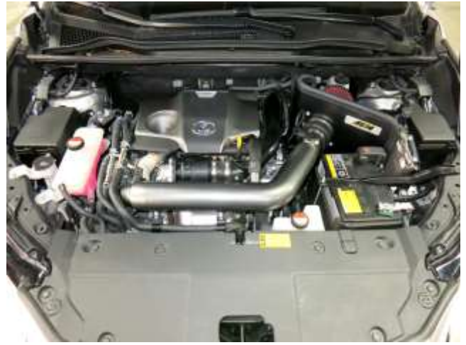
AEM INTAKE INSTALLED
