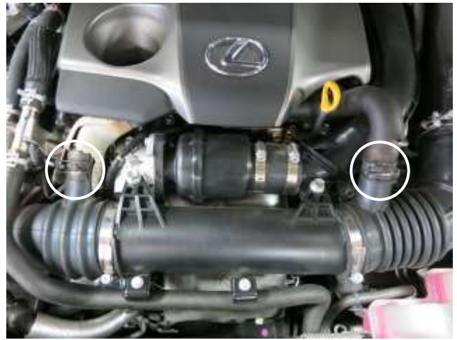
b. Squeeze to loosen the spring clamps and disconnect the vent hoses from the stock intake tube.
