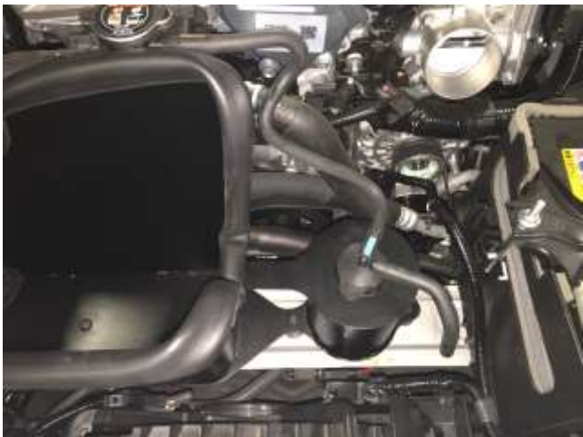
d. Transfer the coolant from the factory tank into the AEM reservoir and seal with factory cap.
