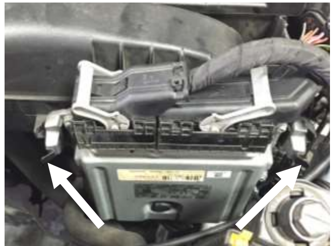
d. Disconnect the ECU mount clips by pushing on them in the direction indicated by the arrows above, then lift the ECU away from the airbox and set aside.
