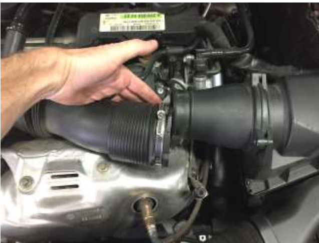
c. Loosen hose clamp at the factory airbox connection and remove as shown.
