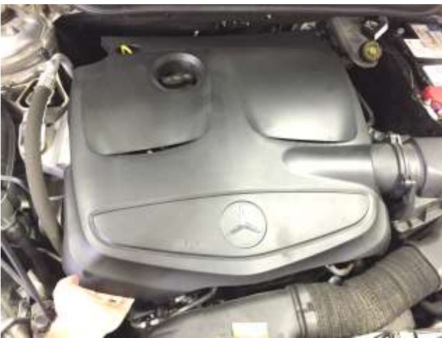
a. Remove engine cover by lifting up at all four corners.
