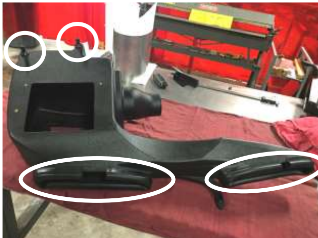
a. Install the airbox mounts on the airbox and trim the supplied edge trim to fit the front air inlets in the airbox.
