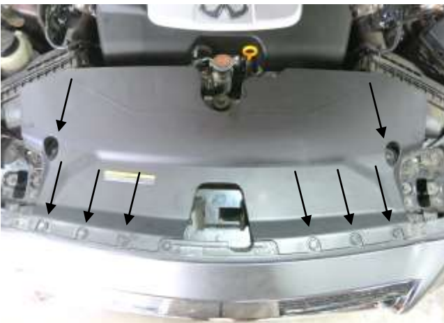
a. Remove the front cover/air scoop by first removing the 8 push-in plastic rivets shown.
