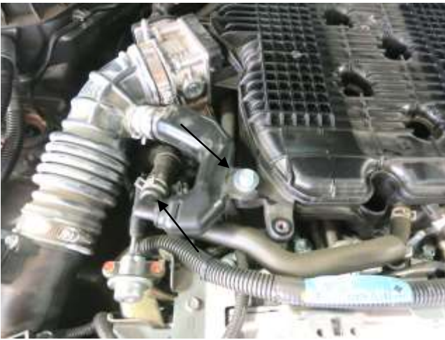
c. Unfasten the passenger side PCV line by removing the bolt shown and disconnecting the hose by releasing the pressure on the spring clamp shown.
