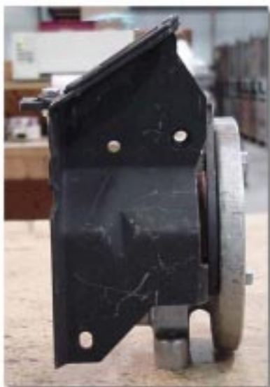
Jeep# 53004278 - This bracket is normally found on Jeep Peugeot transmissions. This bracket mounts to the top of the new linkage bracket.
