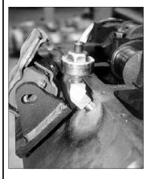
**NOTE:** You may need to grind the small metal tabs located on both sides on your stock 2.8 liter V6 rubber mounts. This may be required to fit the Advance Adapter engine mounts over your stock rubber mounts.
