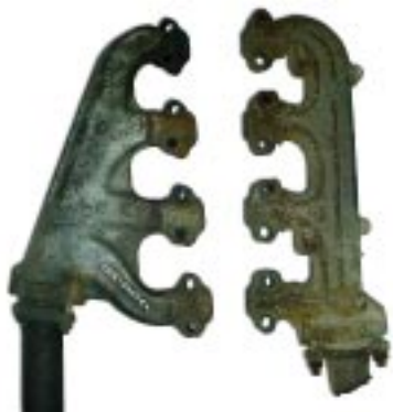
Early stock Ford manifolds that fit with our motor mounts.
