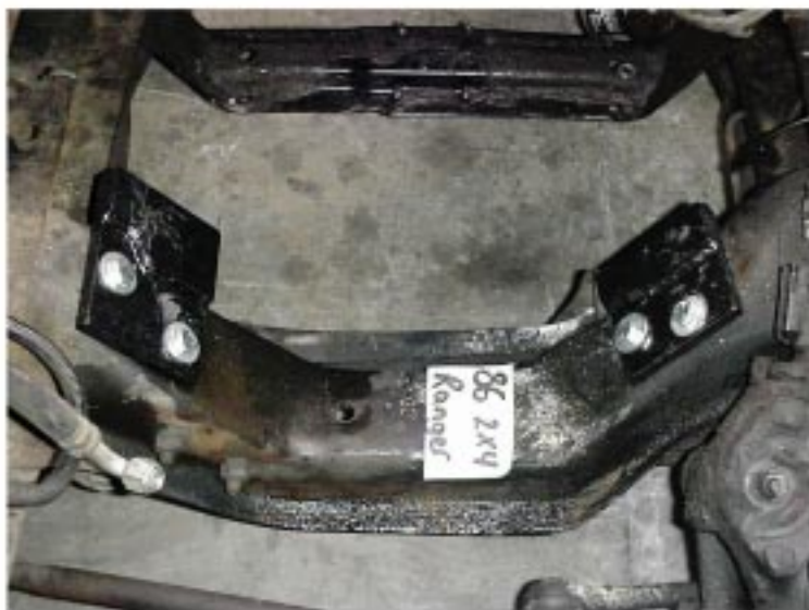
Mounts installed in a Ranger engine cradle
