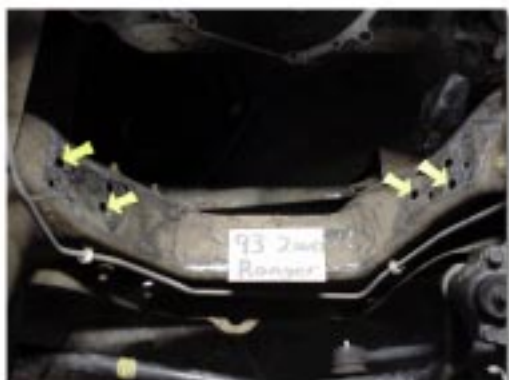
The stock holes on 1993 and newer vehicles are used to mount our mounts.
