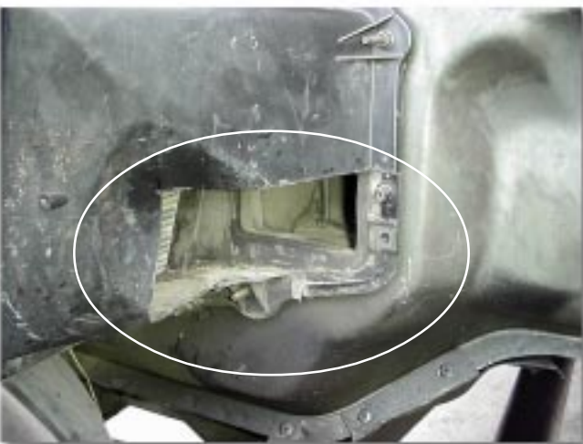
The photo above shows the driver's side firewall modifications.
