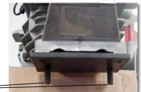
Do not over torque the 7/16 nut to stud on this plate (35 Ft-Lbs Max)
