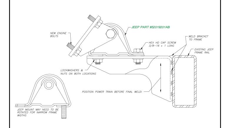
**NOTE**: Vehicles prior to 1980 may require shortening of the frame brackets in order to fit on inside of frame rail.
