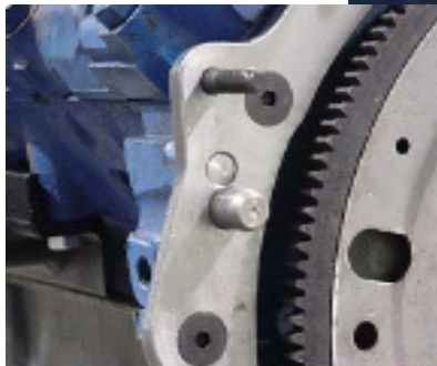
Dowel pin after shortening approximately 1/8".
