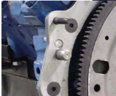
Dowel pin after shortened approximately 1/8".
