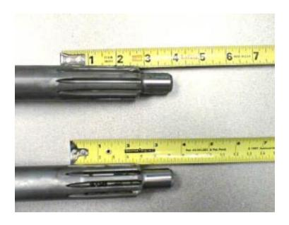
The clutch spline on the lower input shaft is 1/4" to 3/8" shorter than the upper shaft. The splines should be 2-3/4" long to have the proper fit.
