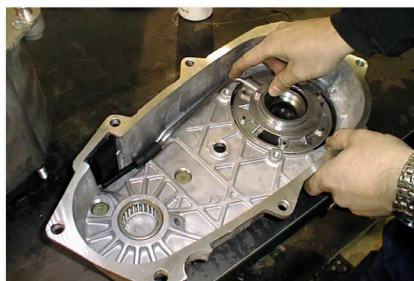
(Fig. 6A) Case Half Pre-assembly
