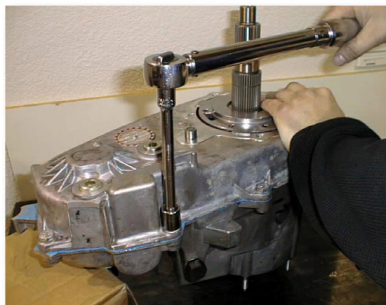
(Fig. 8A) Case Halves Assembled
