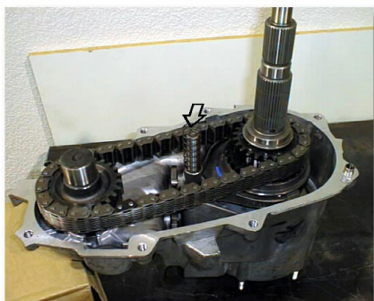
(Fig. 5A) New Main Output Shaft Assembly
