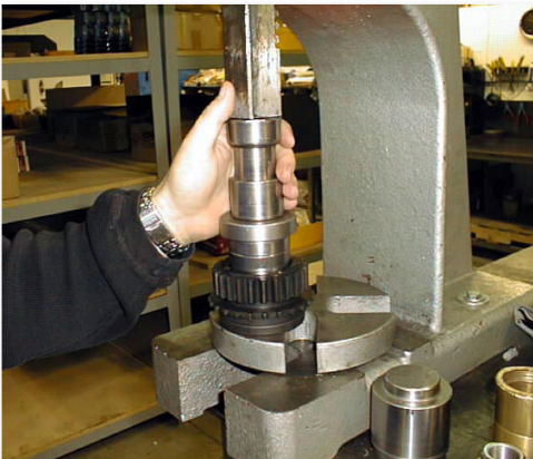
(Fig. 2A) Pull the Needle Bearings Out
