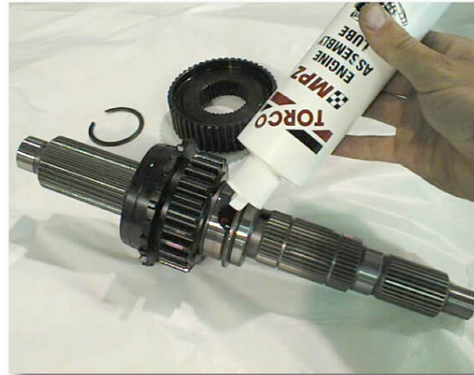
(Fig. 3A) New Main Output Shaft Assembly
