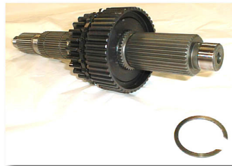
(Fig. 4A) (Large) Retaining Ring Installation
