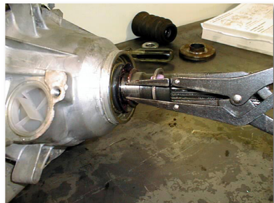
(Fig. 4) Stop Spacer & Snap Ring Removal
