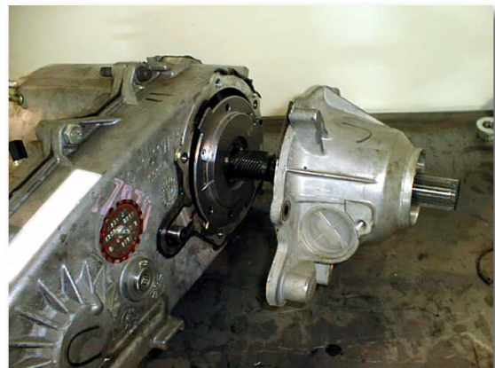
(Fig. 8) Rear Tailhousing Removal
