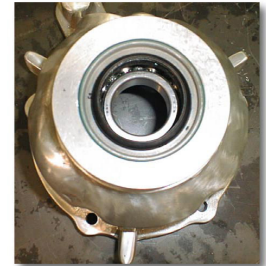
(Fig. 11A) Seal Installed
