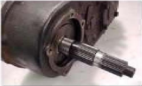
2. Install the shaft through the front of the transfer case, through the slider hub, and onto the stock gear. You should make sure you lube the surface between the gear and shaft. Install the modified thrust washer onto the output shaft. This thrust washer is required to obtain proper gear and slider
