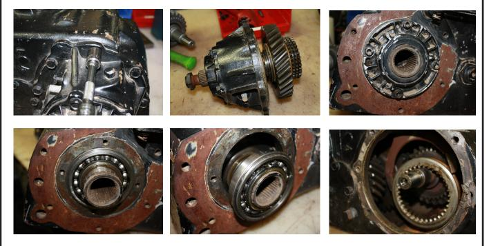
Remove the tailhousing bolts and front retainer bolts (if your transfer case has a front retainer). Shift the transfer case into 2WD high range and remove the tailhousing from the transfer case. Once the T/C output is removed, shift the T/C into low range which will release the slider. Remove the snap ring from the shaft to the bearing so the shaft and the bearing can be separated. This will allow the gear to drop downward and clear the shift fork.
