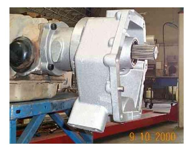
14. Fit the transmission assembly to the transfer case and secure it using the original Toyota bolts.
