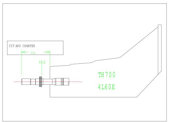
6. **NOTE:** When fitting a six bolt 4L60-E. You will need to fit the six bolt to four bolt adaptor housing to the automatic transmission (part no. MFC1103) before cutting the mainshaft to length. Secure the MFC1103 housing to the transmission using the six M10x1.5x30 socket head cap screws. **NOTE:** Use the original o'ring and silastic to seal the housing to the transmission.
