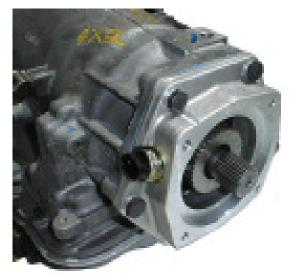
set on the back of the transmission, install the 300619 reluctor sensor into the adapter casting. The 300619 sensor should line up over the teeth of the reluctor clamp. When you obtain this location, remove the adapter housing, making sure not to disturb the position of the clamp on the shaft. With the clamp now exposed, tighten the two set screws on the clamp. Loctite on these set screws is recommended.
