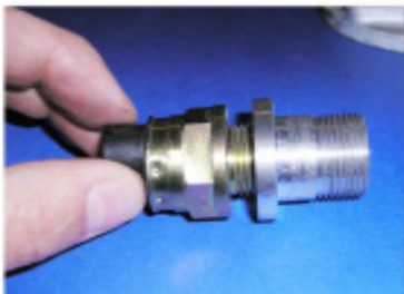
7. Remove the bushing after test fitting and then install the new reluctor sensor.
