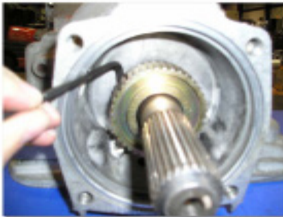
5. Tighten set collar of reluctor ring to lock it to the main output shaft
