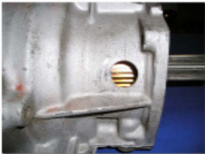
4. Verify that the teeth of the reluctor can be seen through the new hole
