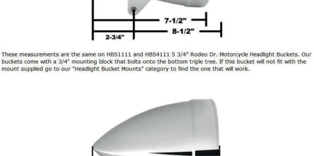
These measurements are the same on HB51110 and HB54110 5 3/4" Rodeo Dr. Motorcycle Headlight Buckets. Our buckets come with a 3/4" mounting block that bolts onto the bottom triple tree. If this bucket will not fit with the
