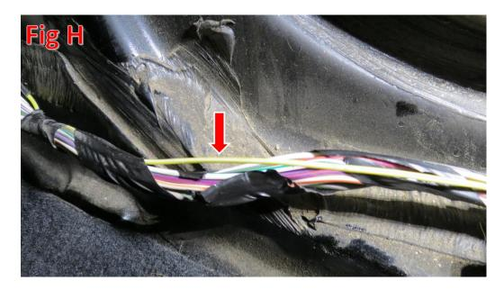
13. Using the splice connector that is already attached to the red LED Harness wire, attach the red harness wire to the Jeep's yellow/white stripe wire. Fig I explains how the splice connector works.
