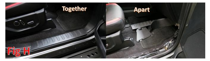
10. Lift the carpet in front of the seat and find the rubber plug. Remove this plug and cut a slit in it for the wiring harness to fit through. Feed the wires through the slit you just cut. Refer to Fig I.
