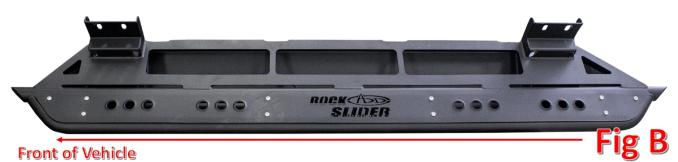
4. Set your ADD Side Step into place on the 6 studs. Secure the Side Steps by either installing the OEM Nuts (x6), or installing the supplied M8 Lock Nuts (x6) and M8 Washers (x6). (Fig C) Install nuts finger tight until they are all installed, then go back and tighten them to the manufacturer's specification.
