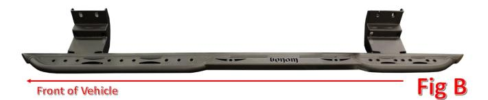
4. Set your ADD Side Step into place on the 6 studs. Secure the Side Steps by either installing the OEM Nuts (x6), or installing the supplied M8 Lock Nuts (x6) and M8 Washers (x6). (Fig C) Install nuts finger tight until they are all installed, then go back and tighten them to the manufacturer's specification.
