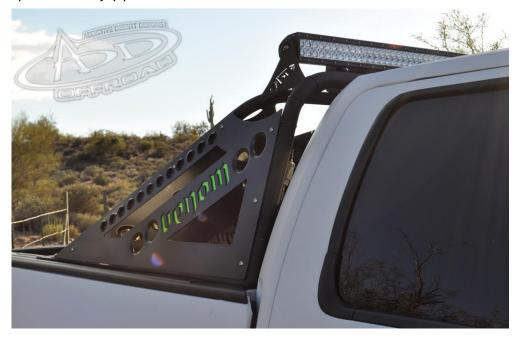
6. Check, and re-tighten if needed, all mounting bolts after 100 miles and periodically thereafter.
