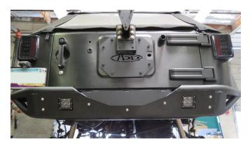
8. Check, and re-tighten if needed, all mounting bolts after 100 miles and periodically thereafter.
