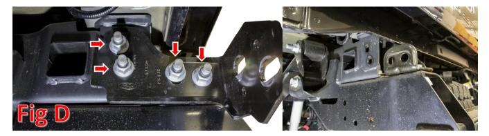
5. Remove the OEM Frame Rail Bracket. Use a 15/16" Socket to remove the two mounting bolts (per side), then remove the bracket. Save these bolts for reuse. (Fig E)
