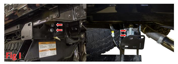
Line up the mounting holes on the back side of your new ADD Bumper with the mounting holes on the newly installed Mounting Brackets. Then, loosely install the supplied 1/2" Bolts (x4), 1/2" Washers (x8), and 1/2" Nuts (x4). (Fig J)
