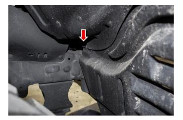
5. If your truck has a one-piece bumper, follow this step. If your truck does not have a one-piece bumper, skip to the following step. Cut your bumper along the body line that separates the two sections of your bumper, but leave a small lip so that you can mock fit the bumper and do your final trimming when you know where the bumper will land. Refer to Fig D.
