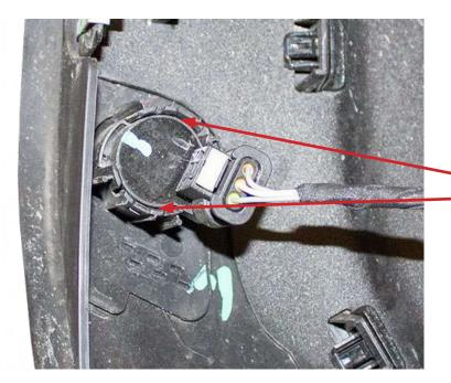
**Spread** these tabs to release the sensor
