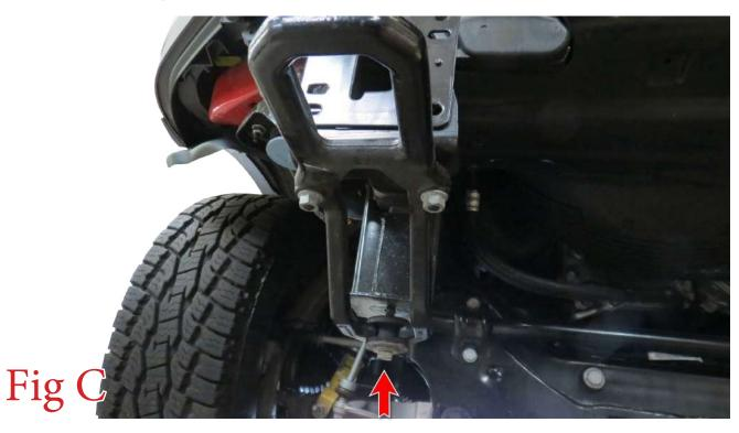
5. THIS STEP IS DONE FOR AESTHETIC REASONS ONLY. IF YOU WISH TO KEEP YOUR TOW HOOKS, PLEASE SKIP THIS STEP. Using a cutoff wheel, or something similar, cut off your frame stilts. Then, grind the area smooth and paint over any bare metal. (Fig D)
