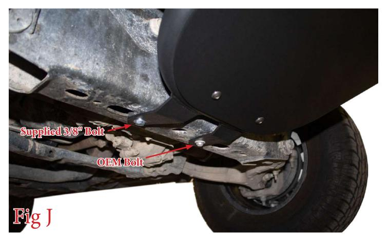
12. Align your bumper so it is straight in relation to the grille/headlights. Then, go back and torque the bolts from Step 10 to 30 foot pounds. Torque the supplied bolt from Step 11 to 25 foot pounds. Torque the OEM Bolt from Step 11 to OEM torque spec.
