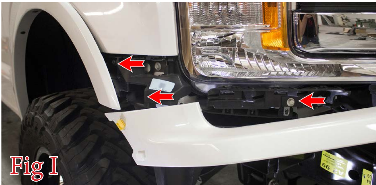
11. Using a 10mm Socket, remove the air dam mounting bolts (x3). Then, remove this air dam from the vehicle (Fig I)
