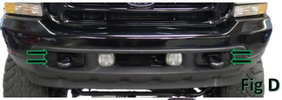
6. Remove the two tow hooks. There are three 15mm bolts holding each of them on. You will need to put new bolts/nuts in the now empty holes. Use the supplied 1/2"x1 1/2" Grade 8 Bolts (x6), 1/2" Grade 8 Washers (x12), and 1/2" Grade 9 Metal Lock Nuts (x6). (Fig E)
